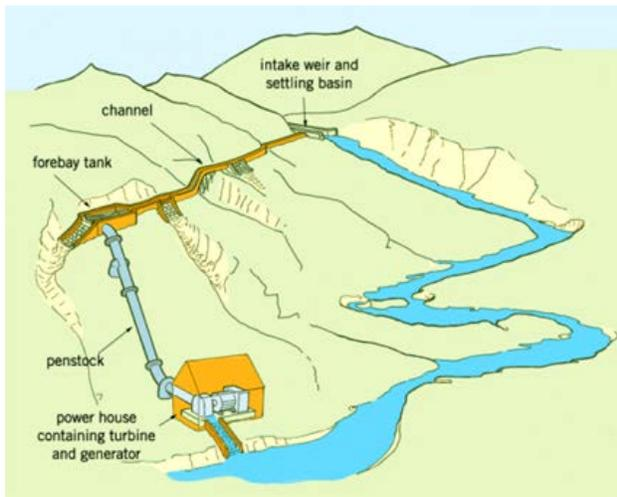
Figure 1: Run-of-river hydro (<http://www.worldwatch.org/hydropower-central-america-renewable-sustainable-and-without-alternatives>)
